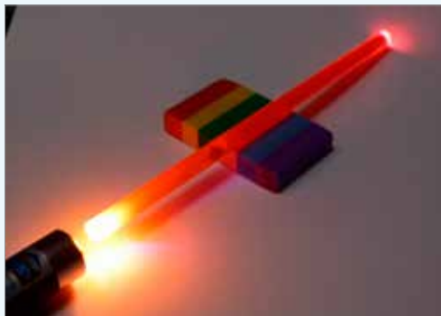
Green laser light causes fluorescence. No laser light emerges from the far end of the rod.
